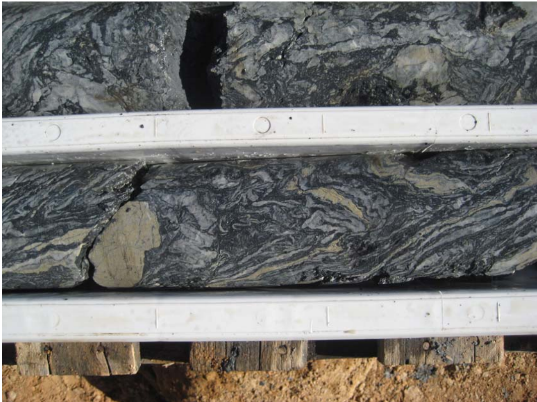
Mylonitic sheared PQ Core (84mm size) in TGA088
