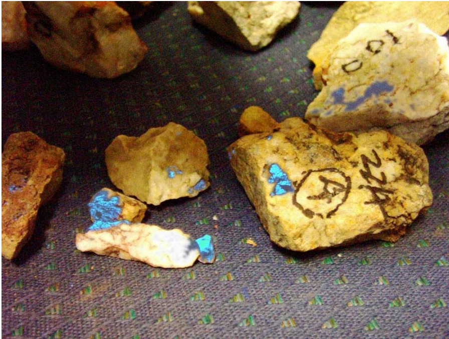
Surface Sample from Whumbal West Showing High Concentrations of Visible Scheelite Under UV Light
