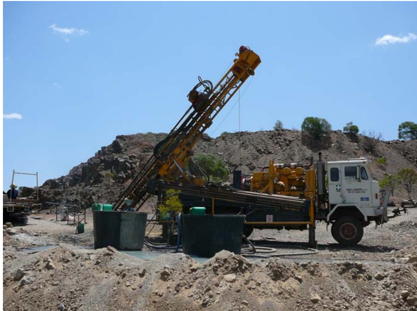
Diamond Drill Rig Drilling Under the Open Pit at Mount Carbine
